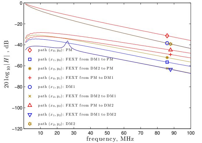
Fig. 3. Example 1. Magnitude responses of direct and far-end crosstalk (FEXT) paths in a 200m 2-pair wireline system with three modes: two differential modes (DM) and one phantom mode (PM).
