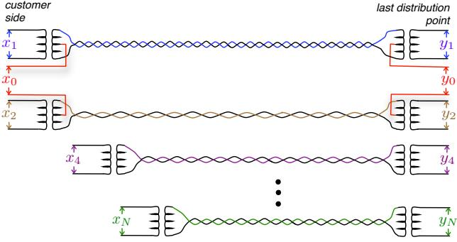
Fig. 2. Example 1. Phantom-mode transmission over two pairs. Two twisted wire pairs can accommodate two differential modes ( $x_1, y_1$ ) and ( $x_2, y_2$ ) and one phantom mode ( $x_0, y_0$ ).  $N = 8$ .
