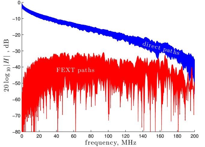
Fig. 6. Example 2. Measured spread of direct paths and FEXT paths in a 24-pair 0.5 mm-cable of 100 m length.
